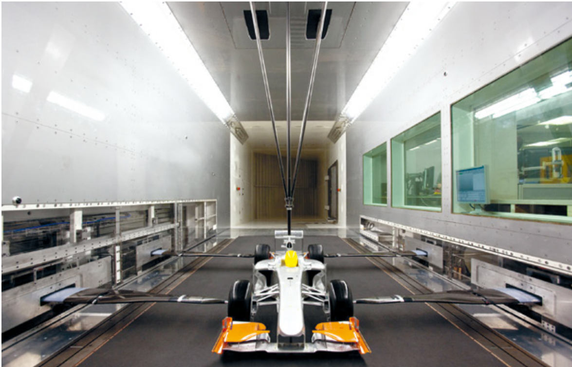
A Lotus F1 model being tested in a wind tunnel. Using 3D printed parts makes it much simpler and faster to test a range of technical solutions.
