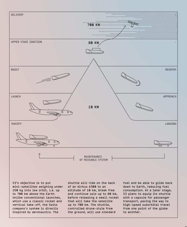
coordinate operations (see the detailed diagram on page 36). S3 will also handle the maintenance of the shuttle, which will be completely reusable and return to Earth after each flight.
