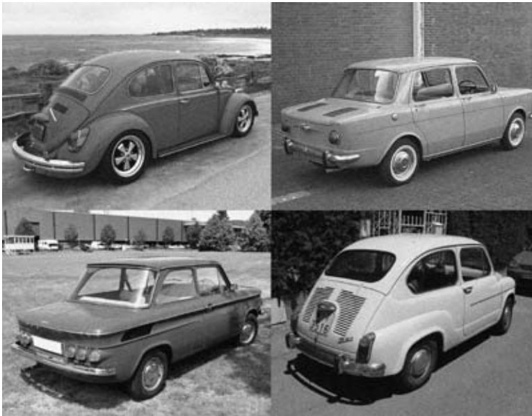
Rear engines had their time of glory before gradually tumbling into oblivion in the 1970s. One notable exception is the Porsche 911 sports car which still features this configuration today. The VW Beetle, Simca 1000 and NSU Prinz and Fiat 600 (above) gained appreciation for their performance on snow compared with traditional front-engine, rear-wheel drive models.
