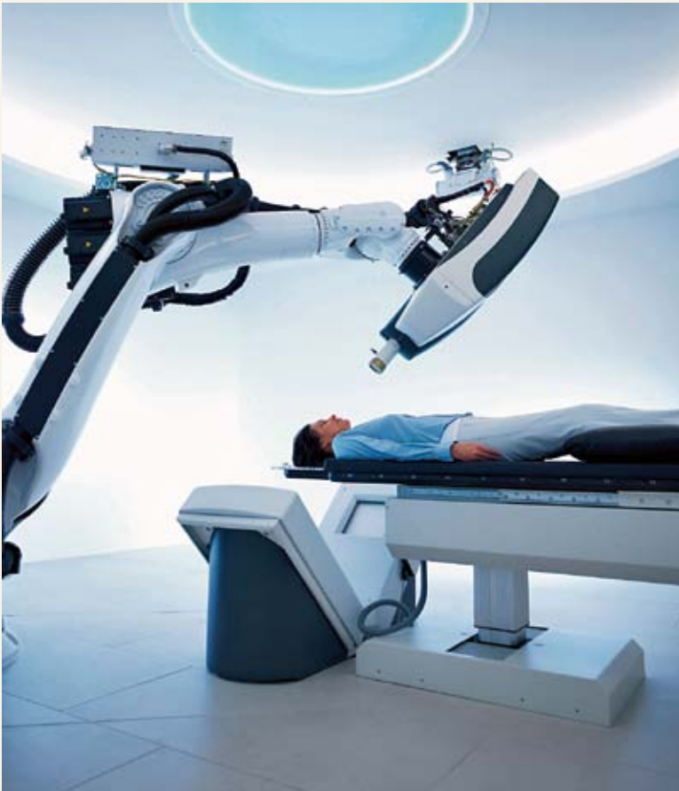
The Cyberknife by Kuka is a robot-controlled radiosurgery system designed to treat solid tumours with sub-millimetre precision.
